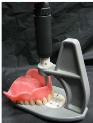
(Figure 2) The Alma Gauge provides precise information when duplicating an existing denture.
