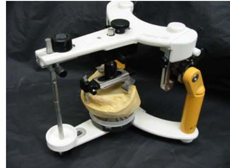
(Figure 3) The horizontal mounting guide produces an ideal orientation of the master cast on the Stratos 200 without a facebow.
